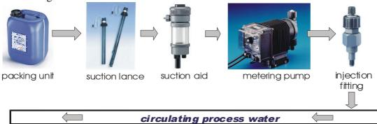
the control of the dosing pump is made by measuring the redox tension of water by a redoxmeasure appliance
